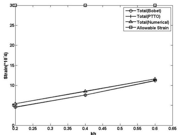
Figure 12. THE MAXIMUM ENVIROMENTAL STRAIN WITH DIFFERENT VALUES OF  $k_h$  AT A DEPTH of 20 M.
