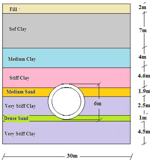
Figure 3. THE PROFILE OF SOIL AND THE TUNNEL COATING.
