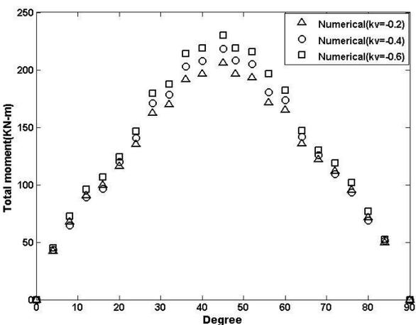
Figure 9. DISTRIBUTION OF THE TOTAL BENDING MOMENT FOR CONSTANT VALUES OF  $k_h=0.2$  AND DIFFERENT VALUES OF  $k_v$  IN 20-M DEPTH.
