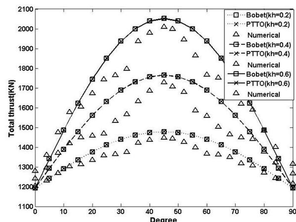
Figure 6. DISTRIBUTION OF THE TOTAL AXIAL FORCE FOR DIFFERENT VALUES OF  $k_k$  IN 20-M DEPTH.
