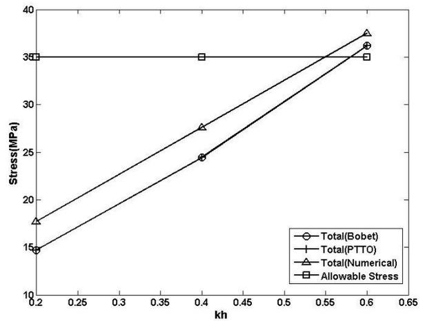
Figure 10. THE MAXIMUM ENVIROMENTAL TENSION WITH DIFFERENT VALUES OF  $k_h$  AT A DEPTH of 20 M.
