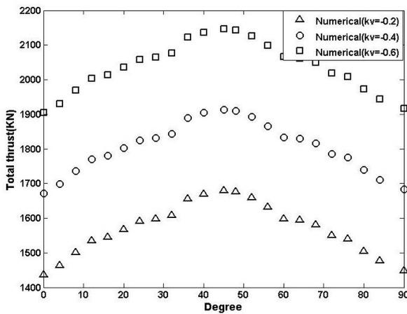
Figure 8. DISTRIBUTION OF THE TOTAL AXIAL FORCE FOR CONSTANT VALUES OF  $k_h=0.2$  AND DIFFERENT VALUES OF  $k_v$  IN 20-M DEPTH.
