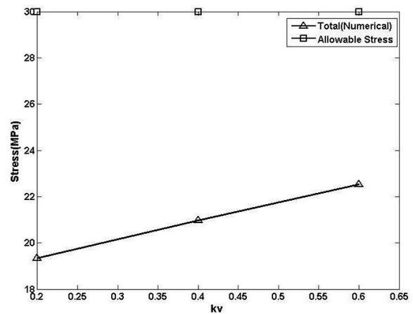
Figure 11. THE MAXIMUM ENVIROMENTAL TENSION WITH CONSTANT VALUES OF  $k_h=0.2$  AND DIFFERENT VALUES OF  $k_v$  AT A DEPTH of 20 M.
