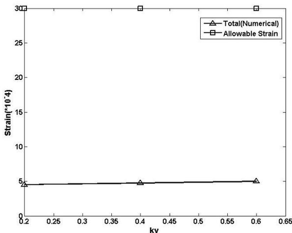
**Figure 13. THE MAXIMUM ENVIROMENTAL STRAIN WITH CONSTANT VALUES OF  $k_h=0.2$  AT A DEPTH of 20 M.**
