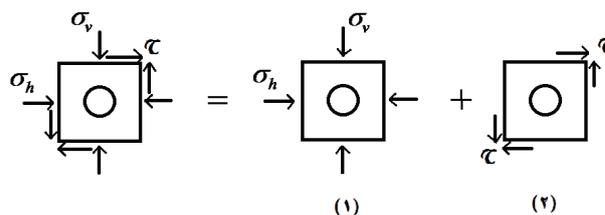
**Figure 1. SCHEMATIC VIEW OF THE PROBLEM LOADING [6].**
