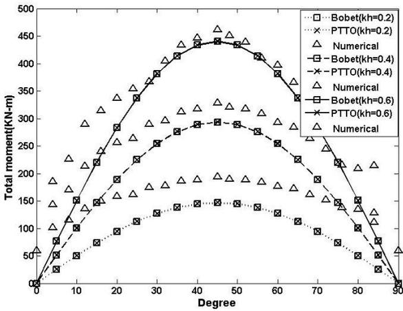
Figure 7. DISTRIBUTION OF THE TOTAL BENDING MOMENT FOR DIFFERENT VALUES OF  $k_h$  IN 20-M DEPTH.
