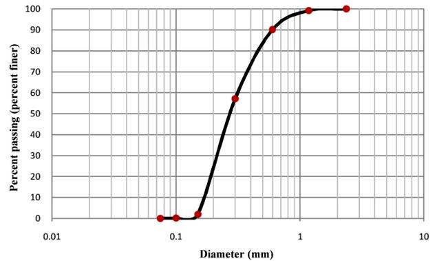
Fig. 3. Grading curves of sandy beach, following the model used in the laboratory
