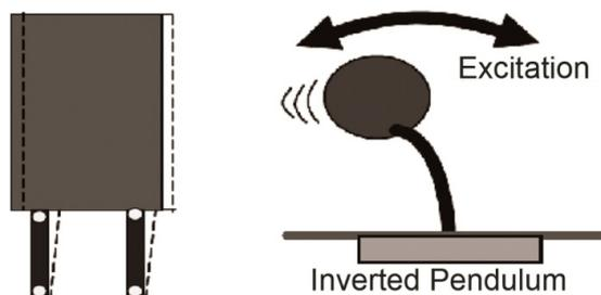
Figure 1: SDOF simulation of soft story (Wibowo et al. 2010)
