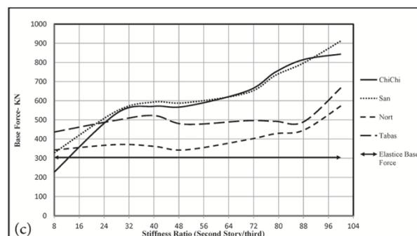
Figure 2: Comparison of the base shears under earthquake records for frames of groups: a) F4A, b) F4B, c) F4C
