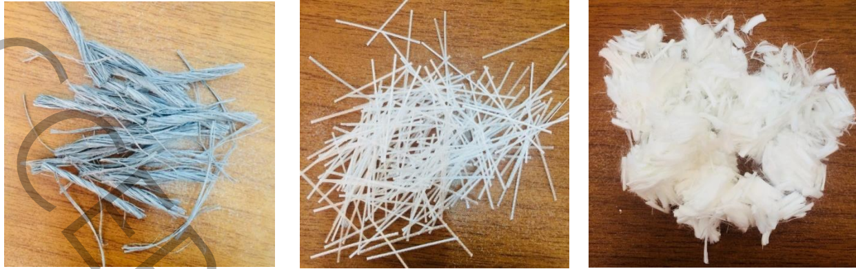
Figure 1. Fibers used in the study (a) Polypropylene (b) Barchip 48 (c) Forta-ferro
