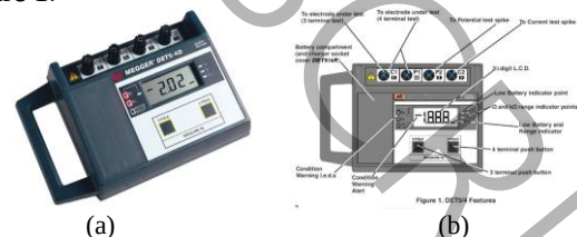
Figure 1. The four-electrode device used to measure apparent electrical resistivity of earth layers, including: (a) 3D view and appearance, (b) introduction of the various components and parts of the device [7]
