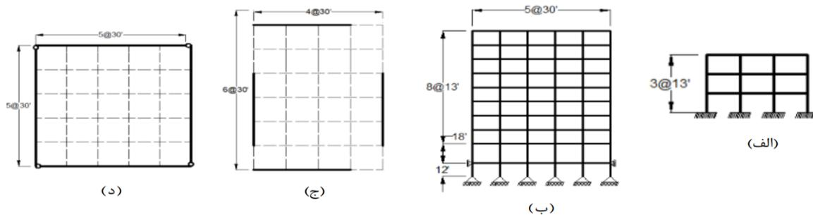
Figure 1. Plans and elevations of 3 and 9 story SAC frames
