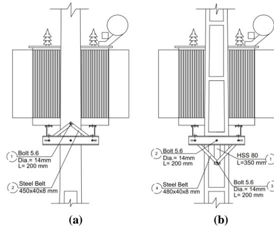
**Figure 2. Retrofit details for the platform-to-concrete-pole connection of the aerial substation: a) connection to the 9 m pole, and b) connection to the 12 m pole**
