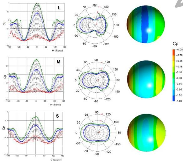
Figure 4: Contour of wind pressure coefficients along with a graph of these coefficients in spherical domes resulting from numerical modeling
