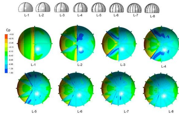
Figure 6: Contour of pressure coefficients on L-shaped spherical domes with protrusions created on the structure
