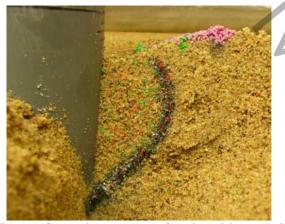
Figure 1. Convective movement of sand particles around the pile [9].
