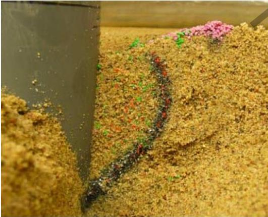
**Figure 1. Convective movement of sand particles around the pile [9].**
