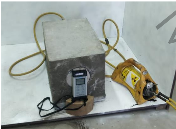
Figure 2. Gamma source, detector, and the condition of the specimen
