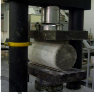
Figure 2 Cylindrical sample in the splitting test
