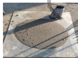
Figure 1. Slump flow test
