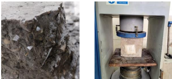
Figure 4. Compressive strength fracture test of cubic specimen with concrete breaker jack, Broken specimen of self-compacting concrete with fiber and iron oxide.
