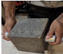
Figure 3. Testing the ultrasonic pulse speed on the test piece.
