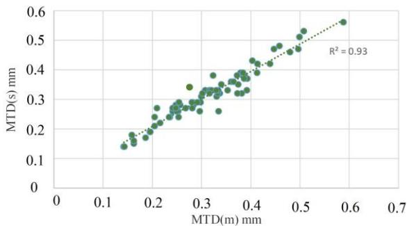
**Figure 2. Correlation between the device and sand patch test results**
