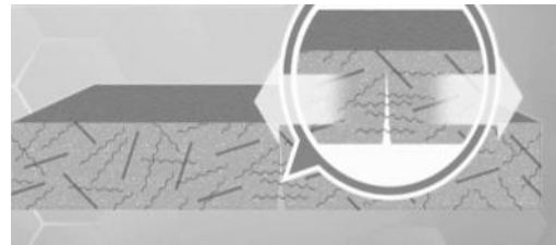
Figure 1. Crack control mechanism by fibers
