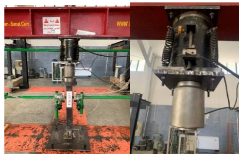
Fig. 2. Loading jack and experimental conditions.
