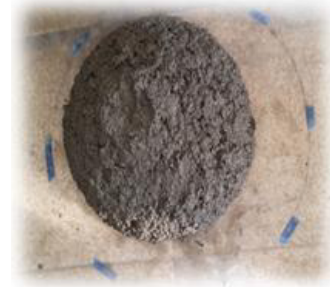
Fig. 1. Slump flow test, sample made based on ICAR mixture design
