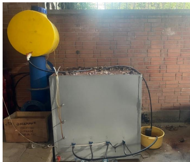
Fig. 2. Semi-industrial system designed for nitrate removal test of the drainage filter
