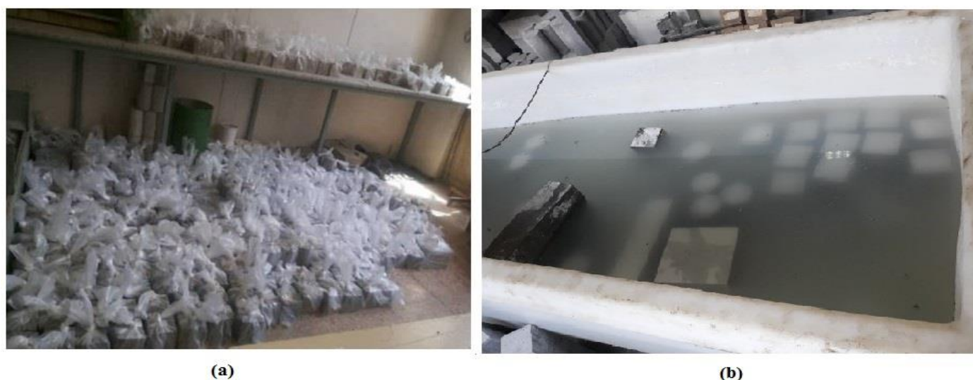
Fig. 1. Curing condition, a) plastic cover curing, b) water curing
