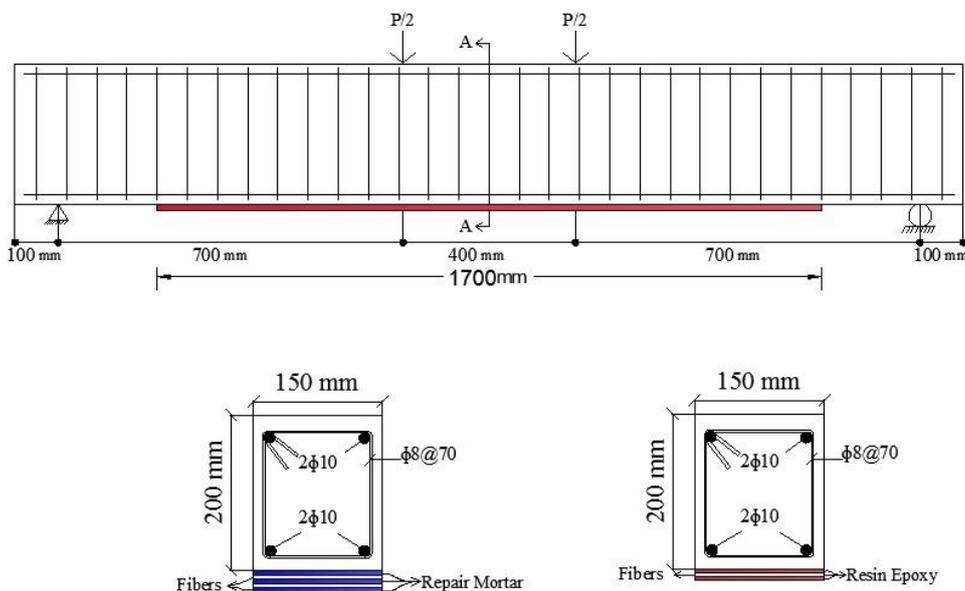
**Fig. 2. The dimension, longitudinal and transverse reinforcement arrangement and the location of the applied loads (the dimensions are based on mm) of (a) the specimen strengthened with CFRP and epoxy resin and (b) the specimen strengthened with CFRP and cement-based mortar**
