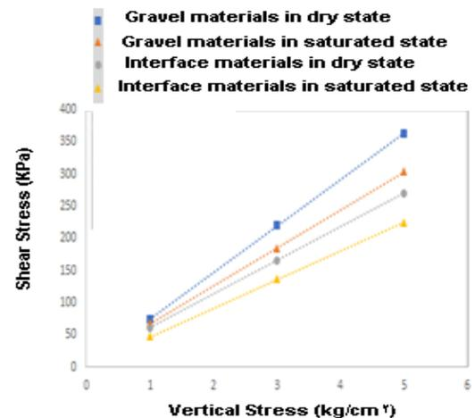
**Fig. 3. Changes in residual shear stress versus vertical stress at 60% relative density**
