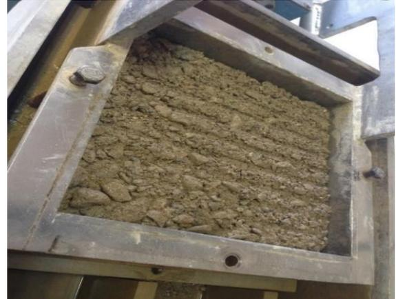
**Fig. 2. Preparation of the filter materials at the lower half of the direct shear box**
