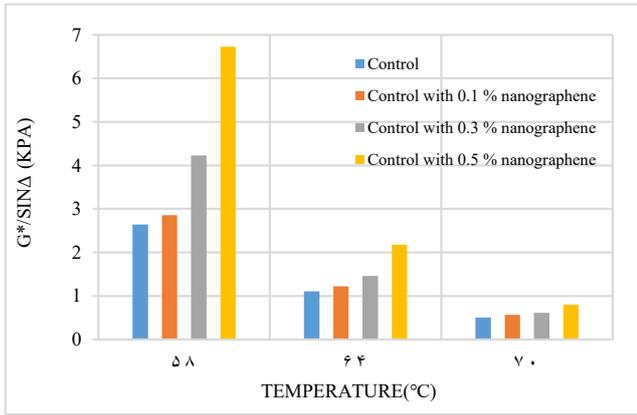
**Fig. 1. DSR test and G\*/Sinδ rutting index results for unaged bitumen**
