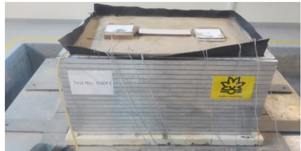
Figure 1. A view of shaking table and laminar shear box
