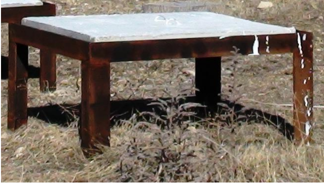
Fig. 1. The setup of blast loading test and arrangement of the support frame
