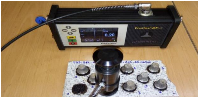
Fig. 1. Pull of Posi Test AT-A apparatus
