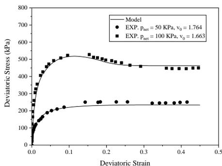
**Figure 3 Comparison of model simulation results with experimental data of unsaturated Kurnell sand under drained triaxial compression loading**
