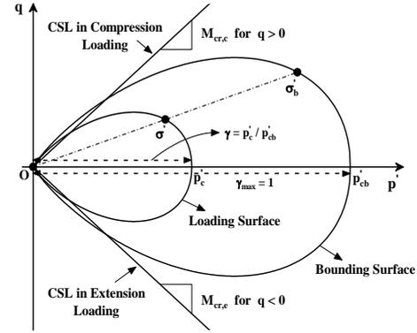
Figure 1 Schematic of the bounding, loading surfaces, and mapping rule, with surfaces size ratio
