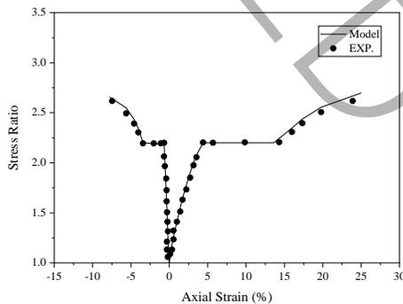
**Figure 2 Comparison of model simulation results with experimental data of unsaturated Pearl clay under triaxial compression and wetting loadings**
