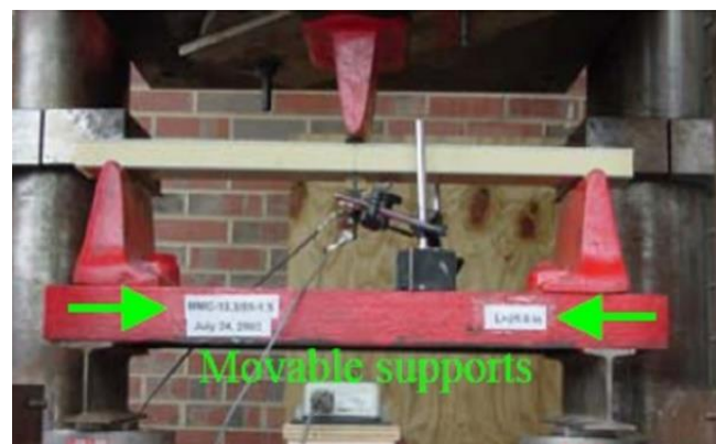
Fig. 2. Three-point bending test on sandwich panels.
