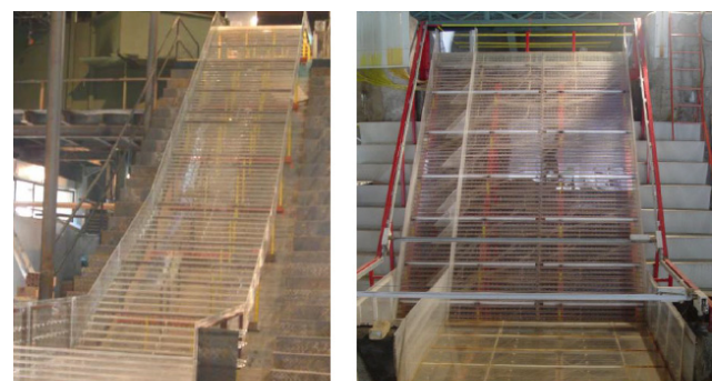
Fig. 1. lower Siahbisheh dam spillway (model D & E) and Zhaveh dam (model F)
