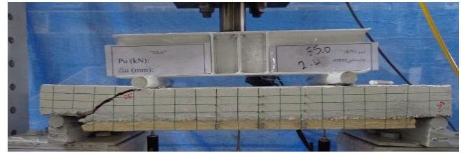
Fig. 9. The failure mode of the WS-L1-Steel
