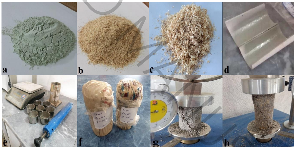
Figure 1. making samples steps - a) zeolite, b) powdered sawdust, c) fibrous sawdust, d) PVC mold, e) compaction test equipment, f) samples' curing process, g) powdered sawdust sample at the moment of rupture, h) fibrous sawdust samples at the moment of rupture
