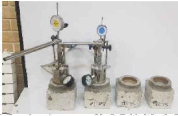
Fig. 1. Concrete specimens prepared for “cylindrical chamber” tests
