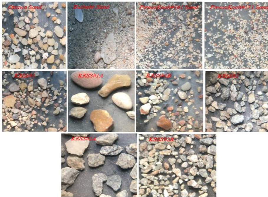
Fig. 2. Sand particles under an optical microscope
