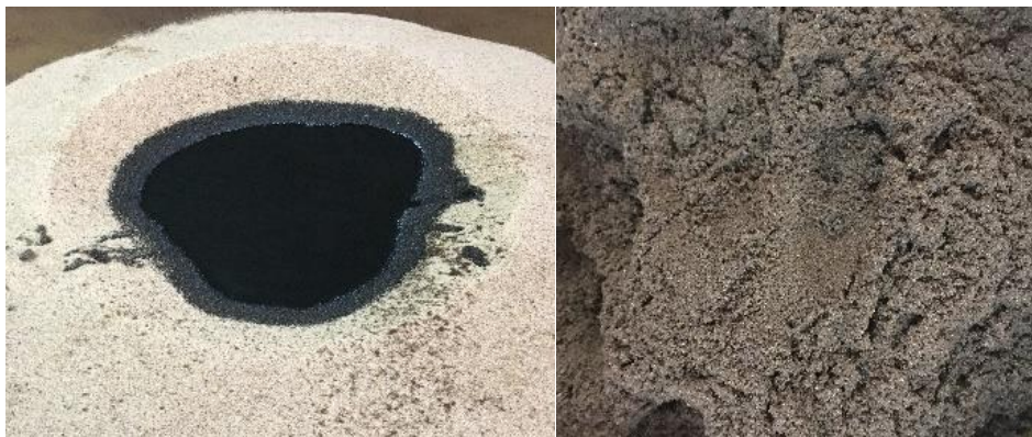
Fig. 3. FiroozKooch#171 contaminated sand preparation
