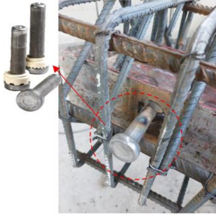
Fig. 1. Details of Shear Studs.
