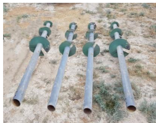
Fig. 2. View of the constructed conical helical pile.
