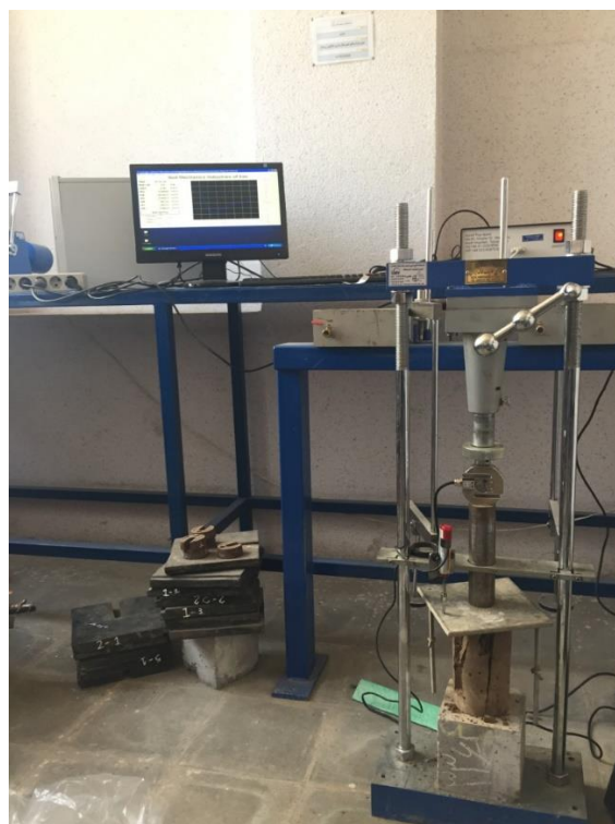
Fig. 1. Field sample test under unconfined compressive strength loading and data recording by data logger.
