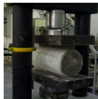
Fig. 2. Cylindrical sample in the splitting test
