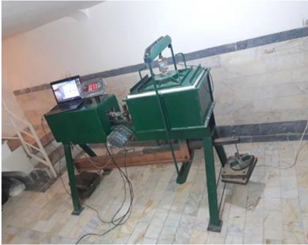
Fig. 1. Geotextile pull-out device
