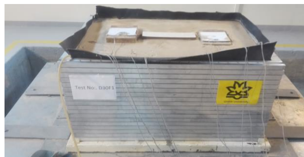
Fig. 1. A view of the shaking table and laminar shear box
