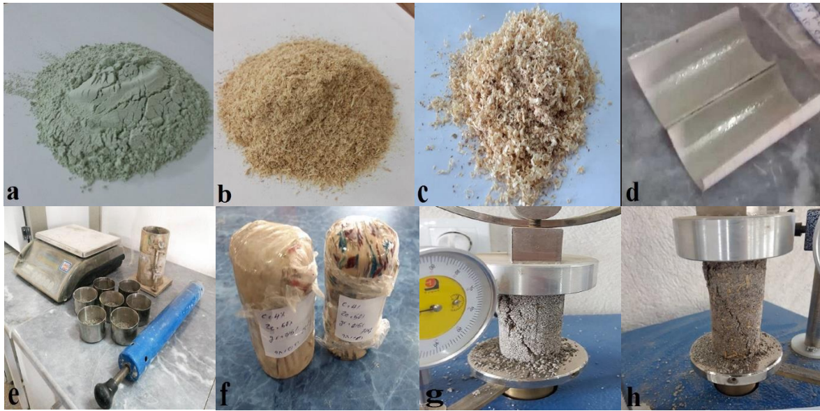
Fig. 1. making samples steps - a) zeolite, b) powdered sawdust, c) fibrous sawdust, d) PVC mold, e) compaction test equipment, f) samples' curing process, g) powdered sawdust sample at the moment of rupture, h) fibrous sawdust samples at the moment of rupture
