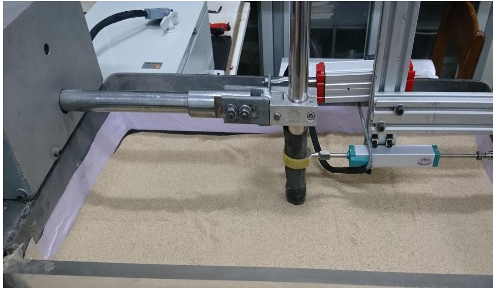
Fig. 1. Experimental set-up for lateral cyclic loading test
