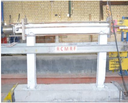
Fig. 1. Model of concrete frame structure without damper
