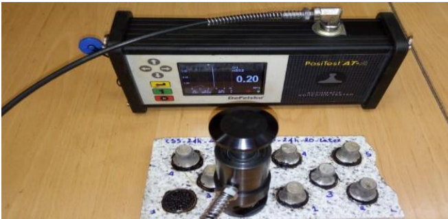
Fig. 1. Pull of Posi Test AT-A apparatus
