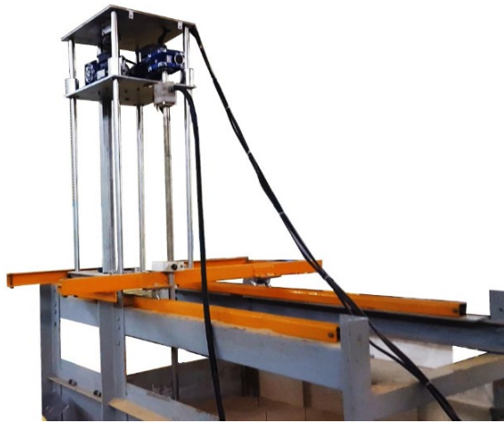
Fig. 1. Micro-jet grouting machine with steel enclosure and its [5] transmission system
