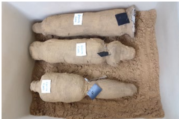
Fig. 2. Columns inserted in the box for curing
