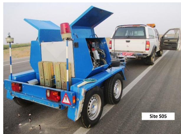
Fig. 1. FWD testing on a site
