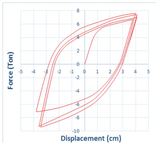
Figure 2. Hysteresis curve of numerical model
