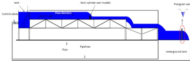
Figure 1: A plan of flume (SCWMRI)
