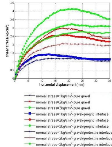
Figure 3. Shear stress- horizontal displacements behavior of gravel samples with 70% compaction degree
