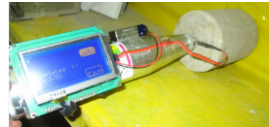
Figure 3. RH impact hammer on the compressed soil
