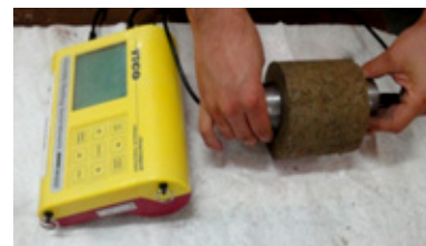
Figure 1. Transmission of ultrasonic waves through the specimen
