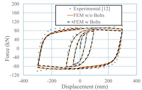
**Figure 4: Hysteresis loops with and without simulation of connecting bolts under longitudinal cyclic loading**
