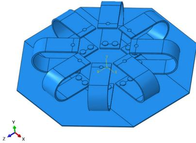
**Figure 8: Circular arrangement of U-plates**
