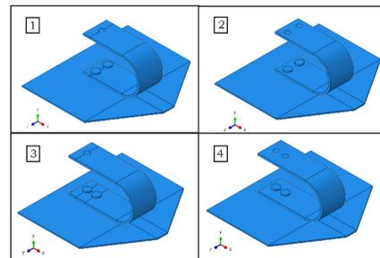
**Figure 6: Four arrangements of connecting bolts**
