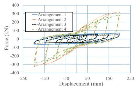
**Figure 7: Hysteresis loops for different arrangements of connecting bolts under transverse cyclic loading**
