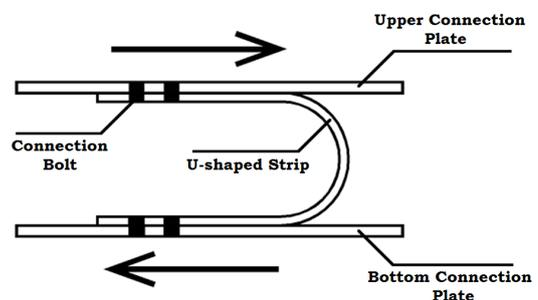
Figure 1: Typical U-shaped damper
