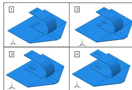
**Figure 6: Four arrangements of connecting bolts**
