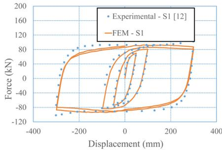
**Figure 3: Comparison between simulated and experimental hysteresis loops**
