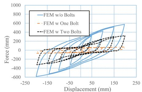
**Figure 5: Hysteresis loops with and without simulation of connecting bolts under transverse cyclic loading**
