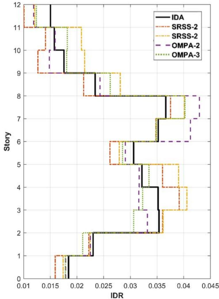
Fig. 2. Inter-story drift profiles of 12 story model.
